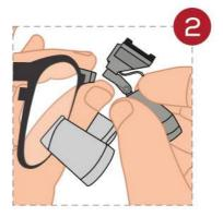
To prevent any damage, carefully detach the light source from the loupes.
